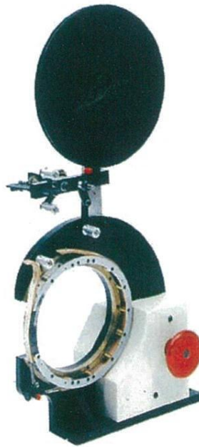
9" Taping and Shielding Head Maximum Coil O.D.: 10.0" (254.0 mm) Minimum Coil O.D.: 2.0" (50.8 mm) Minimum Coil I.D.: 1.0" (25.4 mm) Maximum Coil Height: 3.0" (76.2 mm) Tape Widths: 5/16", 3/8", 1/2", 5/8", 3/4", 1" (8 mm, 10 mm, 12 mm, 15 mm, 19 mm, 25 mm)
