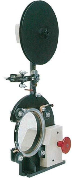
9" SI Taping and Shielding Head Maximum Coil O.D.: 10.0" (254.0 mm) Minimum Coil O.D.: 2.5" (63.5 mm) Minimum Coil I.D.: 0.650" (16.50 mm) Maximum Coil Height: 3.0" (76.2 mm) Tape Widths: 1/4", 5/16", 3/8", 1/2" (6 mm, 8 mm, 10 mm, 12 mm)
