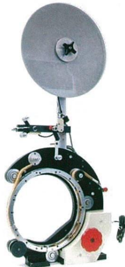
12" SG Taping and Shielding Head Maximum Coil O.D.: 10.0" (254.0 mm) Minimum Coil O.D.: 3.0" (76.2 mm) Minimum Coil I.D.: 1.5" (38.1 mm) Maximum Coil Height: 4.0" (101.6 mm) Tape Widths: 5/16", 3/8", 1/2", 5/8", 3/4", 1" (8 mm, 10 mm, 12 mm, 15 mm, 19 mm, 25 mm)
